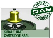
A single-unit cartridge seal is a great advantage for maintenance of the pump as allows the removal and insertion of the seals in less time, having a total guarantee to carry out properly. It 'an **exclusive patent DAB**: a double mechanical seal Sic-Sic with opposite faces, independent from the rotation direction of shaft, with Viton elastomers and leap seal.
